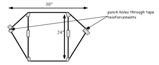
7. Cut a length of string 5 times the length of the dowel rod. Tie the string through the holes using a square knot. Bring the holes together and find the exact midpoint of the string. Tie a knot, leaving a small loop. It is very important that this loop is exactly in the center. If it is not, the kite will not fly straight. Now, tie your flying line in the loop and you are ready to fly!
