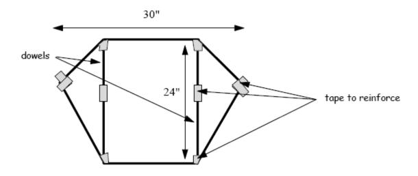
6. After the tape is applied, punch a hole through both corners at the same time. The tape is there to reinforce these corners.
