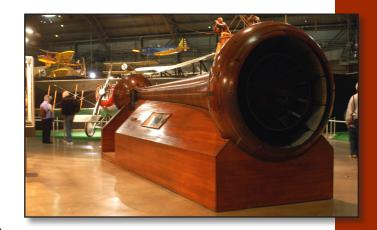
door as air moved over them. During operation, the air was drawn into the small end of the tunnel and exhausted from the large end where the fan was located.<sup>7</sup>
